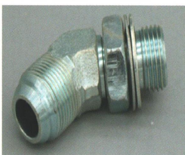
1KG4 45° JIS METRIC MALE 60° CONE/BSP MALE O-RING
