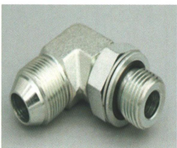
1KG9 90° JIS METRIC MALE 60° CONE/BSP MALE O-RING
