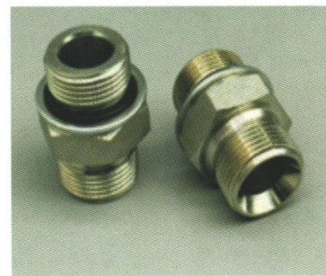
1BH BSP MALE 60° SEATORBONDED SEAL/METRIC MALE O
