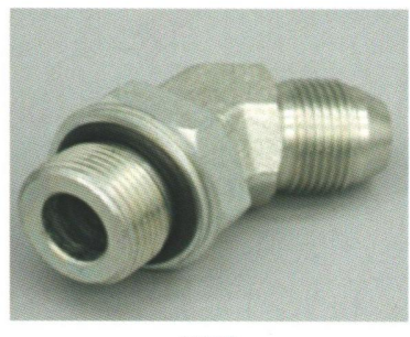
1KH4 JIS METRIC MALE 60° CONE/ METRIC MALE ADJUSTABLE STUD END
