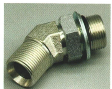
1BO4 BSP MALE 60° SEAT OR BONDED SEAL/SAE MALE ORIN SEAL
